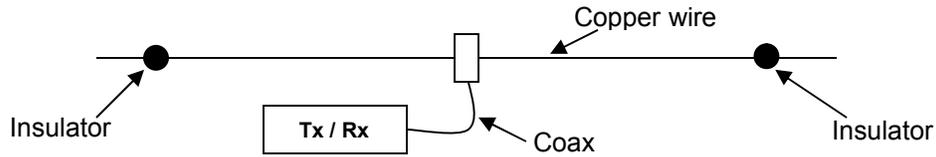
What is the length of the copper wire required for Half Wavelength dipole antenna for 20 meter on frequency 14250kHz?
